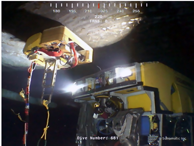
Figure 8: ROV Deployed Subsea Inspection Scanner
