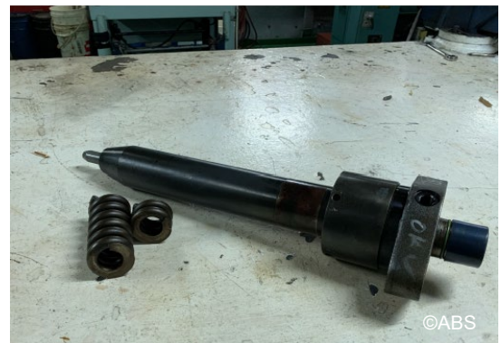
Main engine broken spring for fuel valve found
