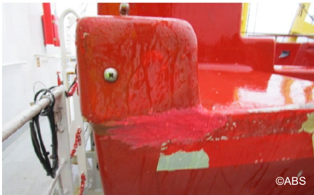
Rescue boat hull minor crack (stern)
