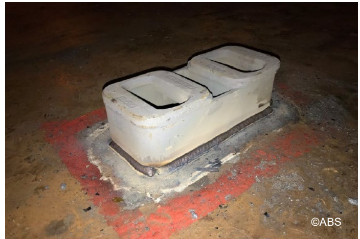
New raised container socket – after
